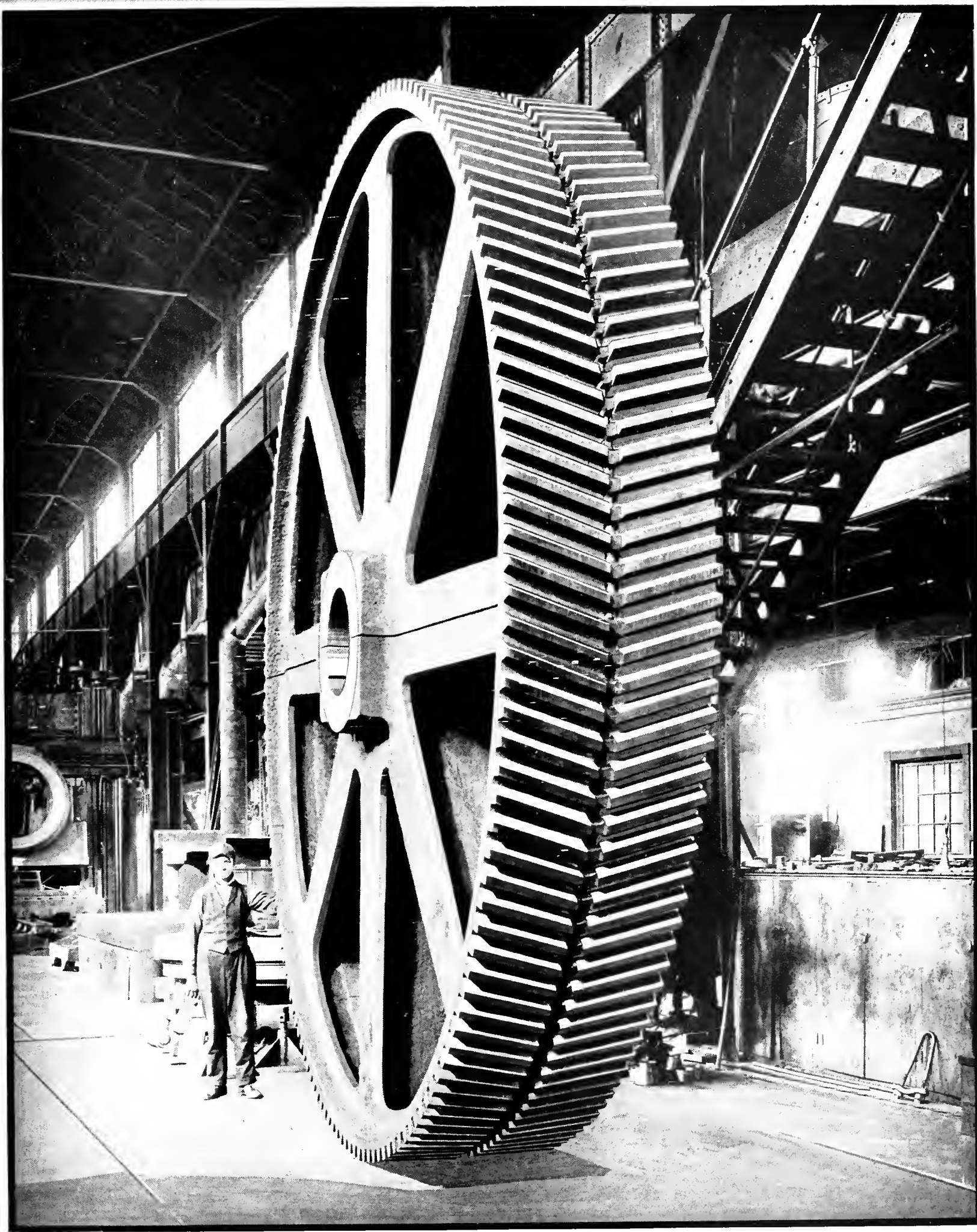
Double Helical Cut Tooth Gear Wheel for 1800 H.P. Gear Drive on Erecting Floor
